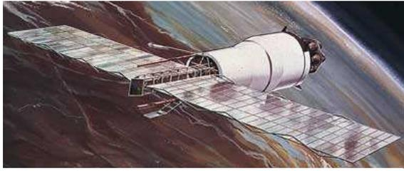
**Figure 2. Pegasus 1 satellite with 180 m<sup>2</sup> micrometeoroid detector (NASA).**
